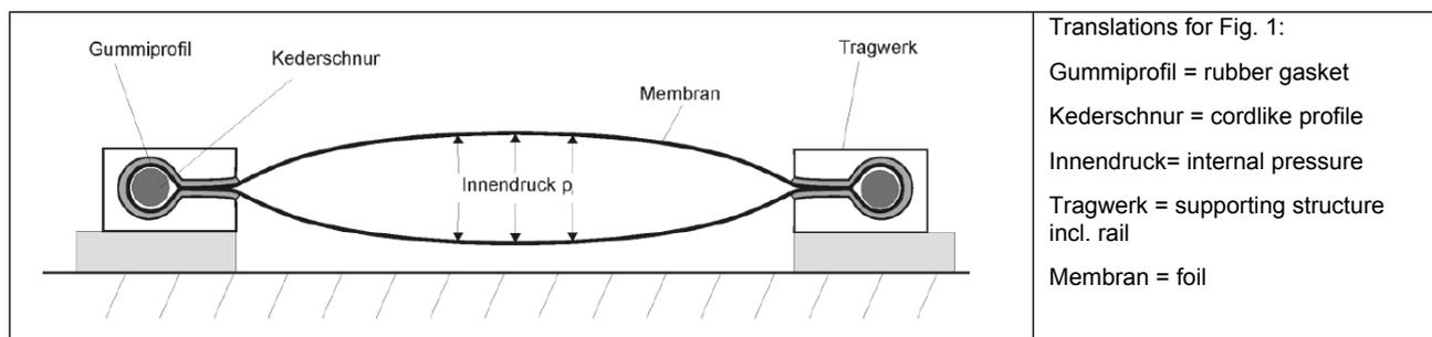
**Figure 1** Cross section of the test specimen (Internal pressure,  $p_i >$  external pressure  $p_a$ )
